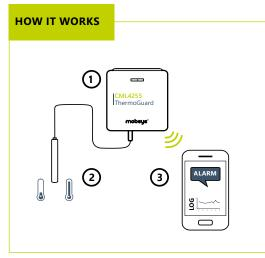
The Mobeye CML4255 continuously measures the temperature values and logs these periodically. In this way you are fully informed about alarm situations and the complete temperature trend.
