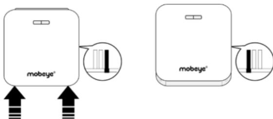
Insert the SIM card into the module.
