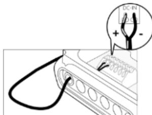
Connect the power adapter (or any other regulated 12-24V DC power supply) to the power input of the connector (press on the green pins to connect the wires).
