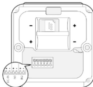
As default the input is programmed as Normally Open (NO) contact. In case the contact is Normally Closed (NC), see paragraph 5.6. To change the delay time before triggering an alarm, see 5.10.
